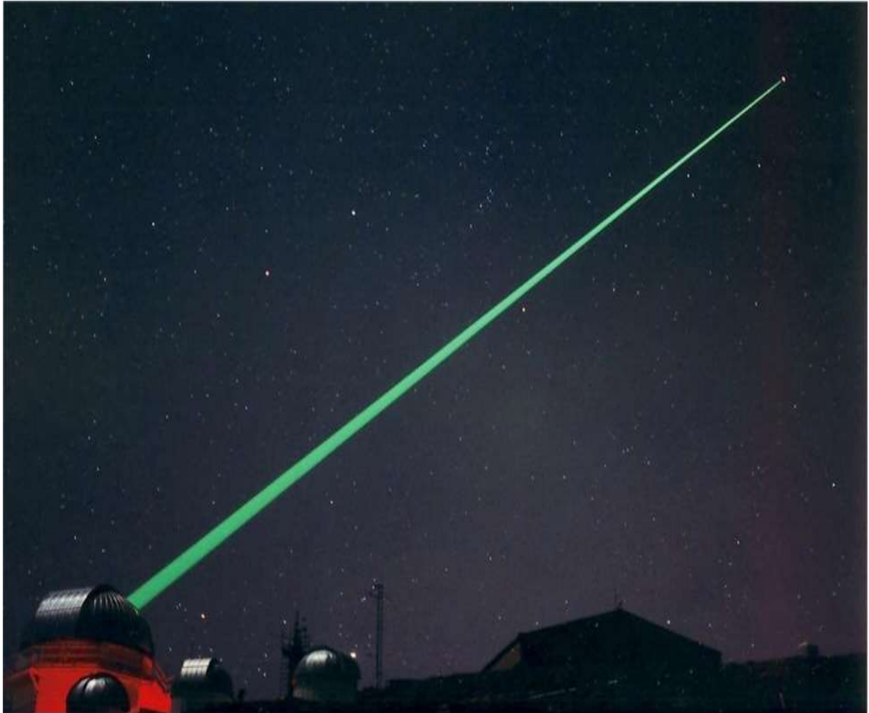
1989, 1.5-m telescope, Starfire Optical Range, Kirtland AFB, New Mexico. First demonstration of continuous closed loop operation of laser guide star adaptive optics.
