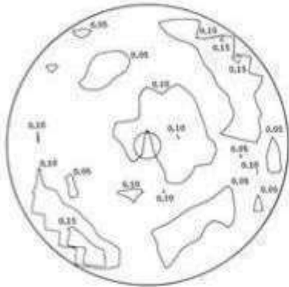
Final surface contour map of 36-inch Mirror (in fractions of wavelength of white light)
